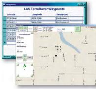
drilling locations (waypoints) are displayed on the screen with a cursor directing the operator's attention to the currently selected waypoint.
