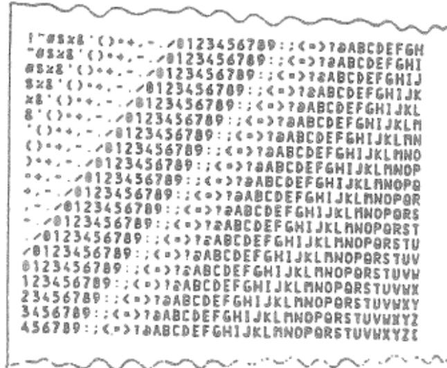
Figure 101. 40 Column Test Pattern
