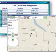
The LogicAll Solutions (LAS) Blast Rig Monitor is an innovative application for excavation equipment which monitors dual GPS receivers mounted to a blast/drill rig and automatically calculates and displays the current location of the drill shaft's center point. Position and distance to the currently selected drilling target are displayed real-time to assist operators to make the most effective and efficient use of the rig. A grid of drilling locations (waypoints) are
